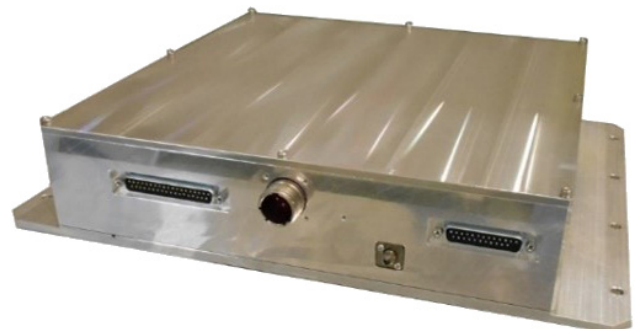
Fig. 3 Appearance of the amplifier
