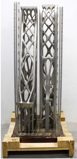
Fig. 6 Two 1500 mm tall jet engine pylons, made of nickel alloy In718, produced within 169 hours
