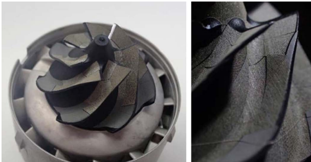
Fig. 5 Riblet processing on a 3D curved surface
