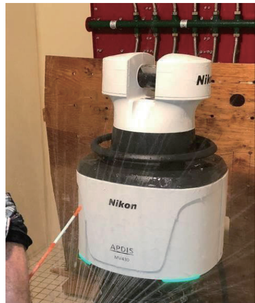
Fig. 12 ADPIS after the IPX4 testing.
